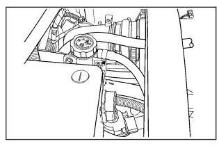
See Engine Compartment Overview on page 373 for the location of the intercooler system pressure cap.
